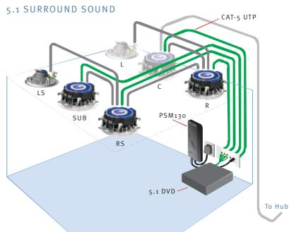
Unique to Systemline Modular, any zone can be upgraded to feature local input 5.1 surround sound by just adding more speakers and CAT 5 cable wired to a Home Cinema Connection Plate within the zone. Just plug in a local source with 5.1 pre-outs and the user can switch seamlessly between local 5.1 surround sound and 6 speaker stereo audio from the Single Source system input.
