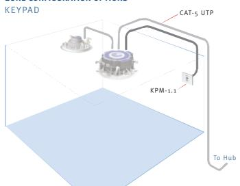
The KPM1.1 Keypad Module can be added to any main zone or sub zone. It enables system input selection, volume, zone on/off and local input (if fitted). It also features a built-in IR sensor.
