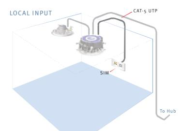
Installing a SIM module and running a CAT-5 cable to the SLM2 within the zone permits a local audio source to be played as well as the main system audio source. Simply connect a local source to the SIM and select using the 'L' button on the remote control or from the keypad.
