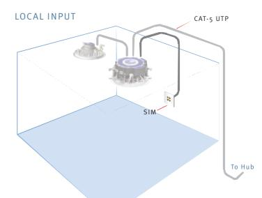
Installing a SIM module and running a CAT-5 cable to the SLM2 within the zone permits a Local audio source to be played back as well as the main system audio source. Simply connect a local source to the SIM and select using the 'L' button on the remote control or from the keypad.
