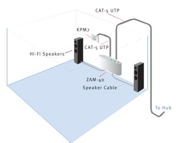
The Zone Amplifier Module (ZAM-40) provides similar functionality to the SLM2 in-ceiling speakers, but allows a wider choice of speakers - from passive in-ceiling, in-wall to free-standing hi-fi speakers. The ZAM-40 connects to the Hub in much the same way as the SLM2 speakers, but it has stereo outputs for powering external speakers using conventional speaker cable. It can also be upgraded to provide a higher output by connecting a PSM130. The KPM7 keypad may also be connected.
