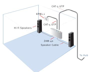
The Zone Amplifier Module (ZAM-40) provides similar functionality to the SLM in-ceiling speakers, but allows a wider choice of speakers - from passive in-ceiling, in-wall to free-standing hi-fi speakers. The ZAM-40 connects to the Hub in much the same way as the SLM speakers, but it has stereo outputs for powering external speakers using conventional speaker cable. It can also be upgraded to provide a higher output by connecting a PSM130. The KPM1.1 Keypad may also be added.
