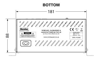
\*All measurements in mm \*\*Grey dimensions apply when product is fitted with wall brackets
