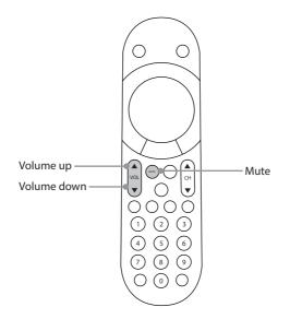
8.1 There are no direct codes for this remote, the setup is done inside the Sky Q box menu. Select *Philips* as the manufacturer. You are then given 33 possible options and just have to work through them until the Touch remote controls the volume on the soundbar. It normally works on *option 7*.
