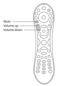
7.1 Turn the S7 zone onto a local source with a LIM and IR receiver and turn the volume up.
