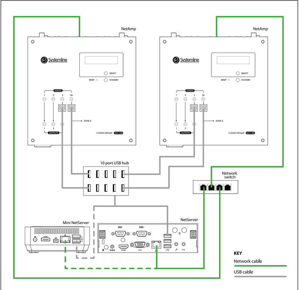
*Please note: It is important that you connect the USB cables and switch the NetAmps on before the NetServer when first installing.*
