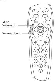
When in TV control mode, the handset will allocate some additional IR functions as shown below:
