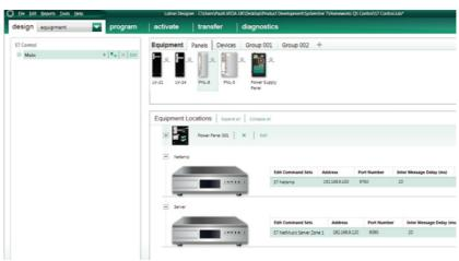
2.5 Add a command set for NetAmp and enter the commands for both zones 1 and 2, making sure you check the box  $Use\ RS232\ terminator$  and select  $<\!CR\!><\!LF\!>(0D\ 0A)$  and select ASCII data type. You can copy the commands from Appendix 1 at the end of this document.
