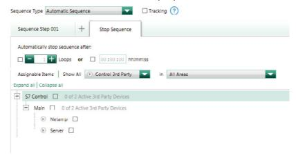
Set up the volume button as *Dual Action* type, starting the volume sequence on press, and stopping it on release.
