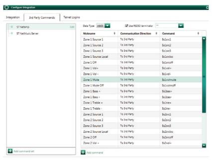
2.6 Add a command set for the S7 NetServer for zone 1, each zone requires its own unique set of commands which includes the unique MAC address of the zone. This MAC address can be obtained from the NetAmp web page. Source 3A corresponds to zone A, source 3 corresponds to zone B. You can copy this address and edit the list of commands from Appendix 2. Make sure you tick the check box *Use RS232 terminator* and select *<CR> <LF>* (*OD 0A*) and select *ASCII* data type.
