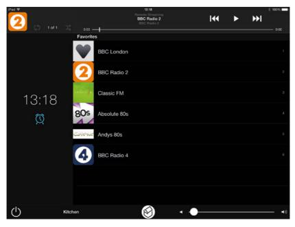
In order for the Lutron system to select a favourite in a zone, it must communicate with the server and also the NetAmp controlling the zone. To adjust the volume, the QS system need only send a command to the NetAmp.
