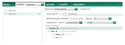
You should set up just one step with the volume command and select the box *Automatically go to the next step after* and set it at 1s. Uncheck *Tracking* and set up the Stop Sequence without any commands, but remove the check for *Automatic stop sequence*.
